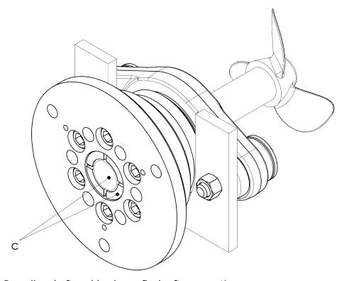
Fig. 6-6 Propeller shaft and bush are flush after mounting
