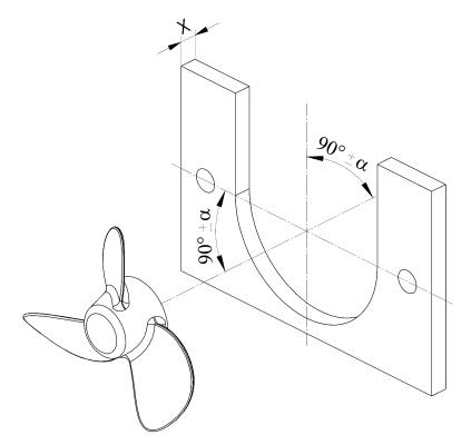
Fig. 6-2 Installation angle of the bearing
