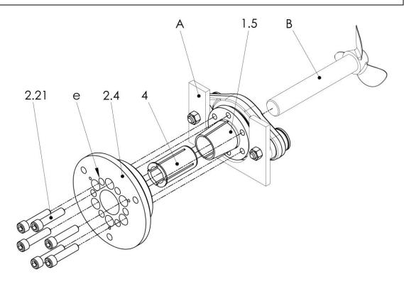
Fig. 6-4 Mounting the hub
