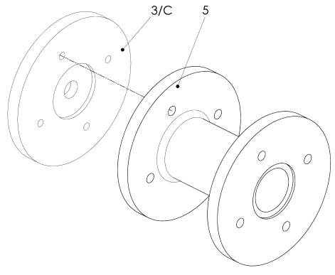
Fig. 6-8 Mounting the adapter (5; if necessary)
