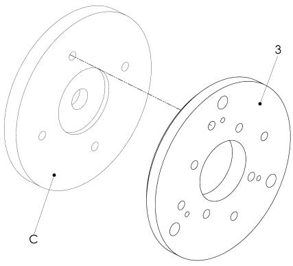
Fig. 6-7 Mounting the adapter (3)
