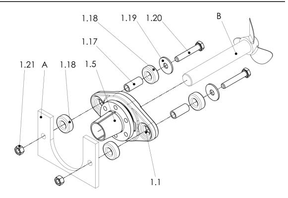
Fig. 6-3 Mounting the bearing to the bulkhead (CENTA-TB-2)
